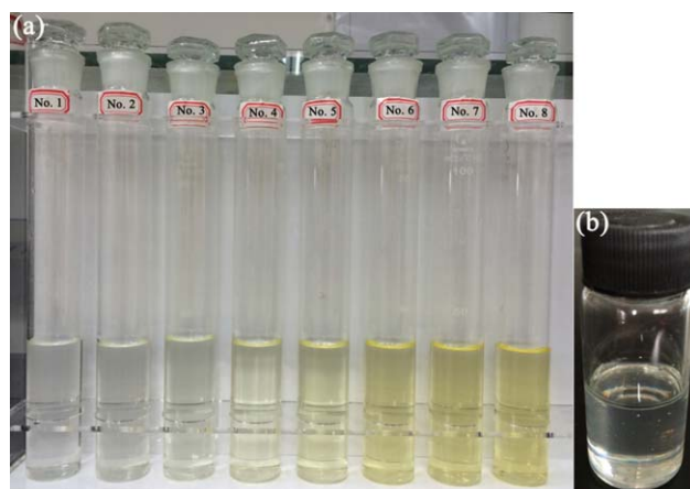
Figure 4. The appearance of BPEFPGMA: (a) Gardner scale from No. 1 to No. 8; (b) BPEFPGMA. [Color figure can be viewed in the online issue, which is available at wileyonlinelibrary.com.]
